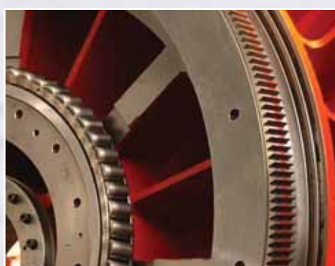
Dettaglio cuscinetto centrale corona dentata Detail of the roller bearing crown-gear
